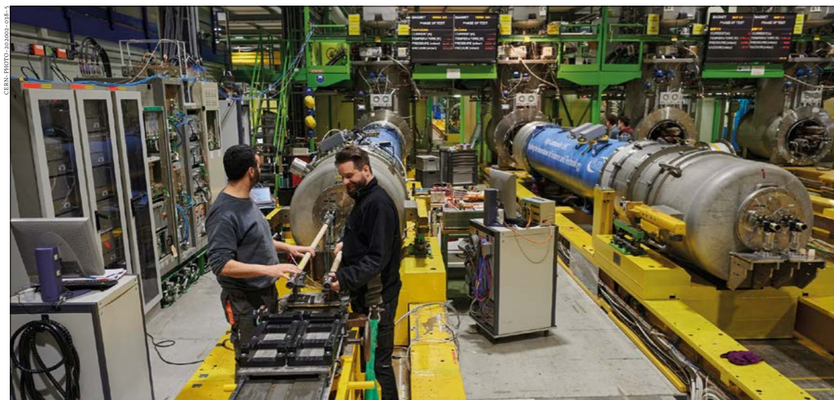
Power couple Nb 3 Sn 11 T dipoles for the HL-LHC undergoing tests at CERN's SM18 facility in February.
