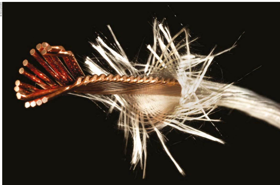
Wired A Nb 3 Sn cable, showing the single strands and the glass-fibre insulation, partially unwrapped.
