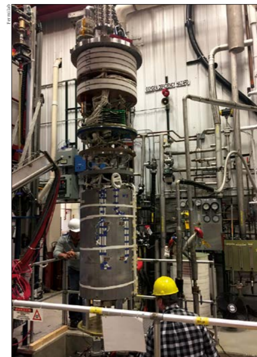
Cos-theta 1 The MDP “cos-theta 1” dipole accelerator magnet at Fermilab, which achieved a field of 14.1 T (the highest ever achieved for such a device at an operational temperature of 4.5 K) in 2019.
