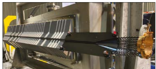
Fig. 1. Half of the SMOG2 storage cell (black), attached to its wake-field suppressor (black, right) and the VELO RF foil (grey, left).
