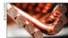
On the cover: Composite Cu/Nb 3 Sn multi-filamentary strands (1 mm diameter) for new accelerator magnets. 34
